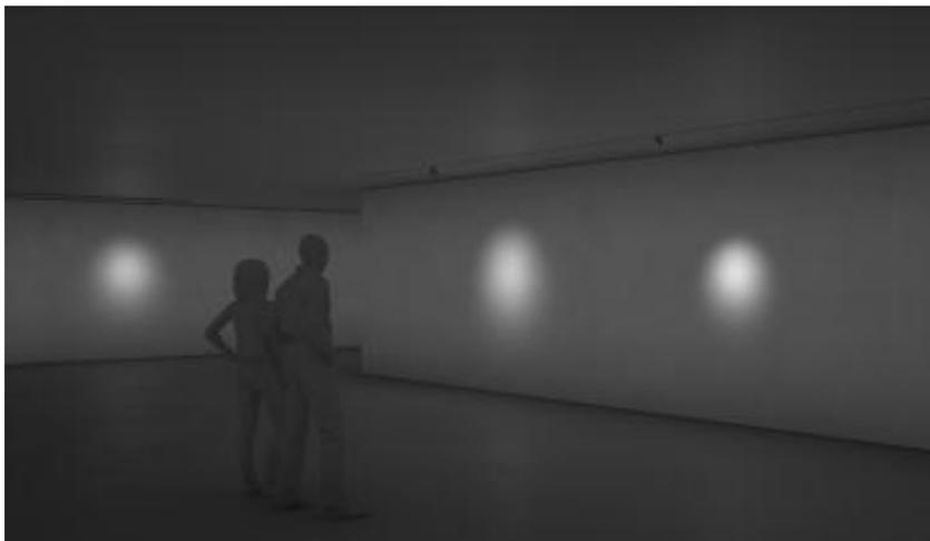
**Fig. 5:** Visualization SUPERSYSTEM spot size 65 mm, 65 mm, 45 mm, 25 mm recessed surface mounted.
